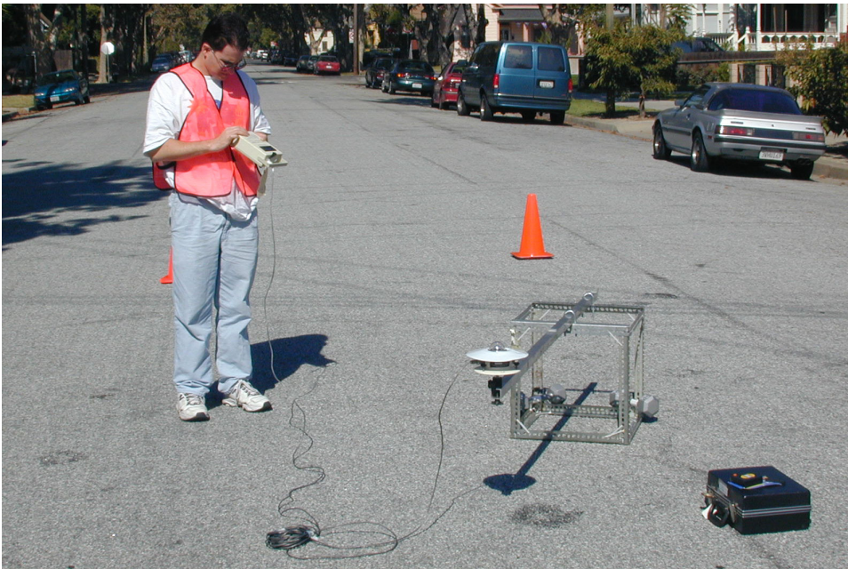
Dr. Ronnen Levinson taking reflectance measurements in San Jose. Photo: Lawrence Berkeley National Lab
